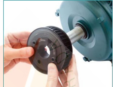
INSERT SCREWS AND LOCATE ON SHAFT
