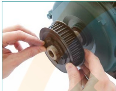
TIGHTEN SCREWS FINGER TIGHT
