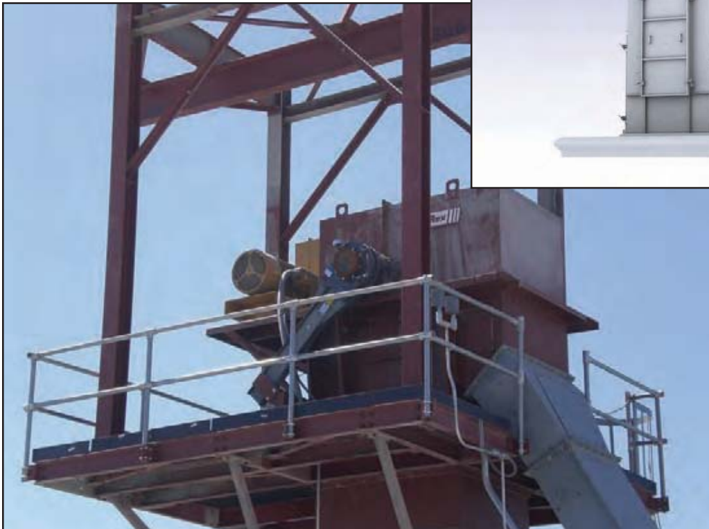
Rexnord Super Capacity elevators can be designed and built with large platforms and hoist frames that allow for easy maintenance access.
