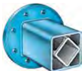
Fig. 9 Flange welded on housing
